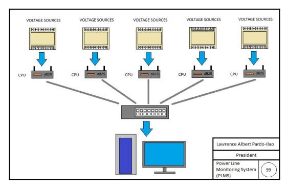
In this example, we are monitoring  $5/\text{cpu} \times 5 = 25$  inputs or Solar Array to be monitored.
